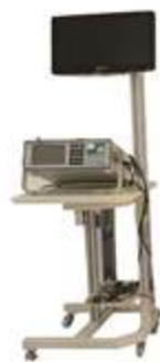
Power grid simulation equipment set for relay protection practice
